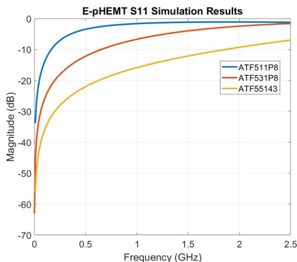
Fig. 2. S11 simulations of E-pHEMT devices as a function of the modulation frequency
