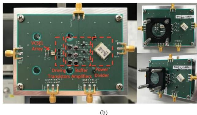
Fig. 3. VCSEL array transmitter – (a) schematic of distributed current VCSEL array driver, (b) fabricated transmitter PCB with and without a collimation lens mounted
