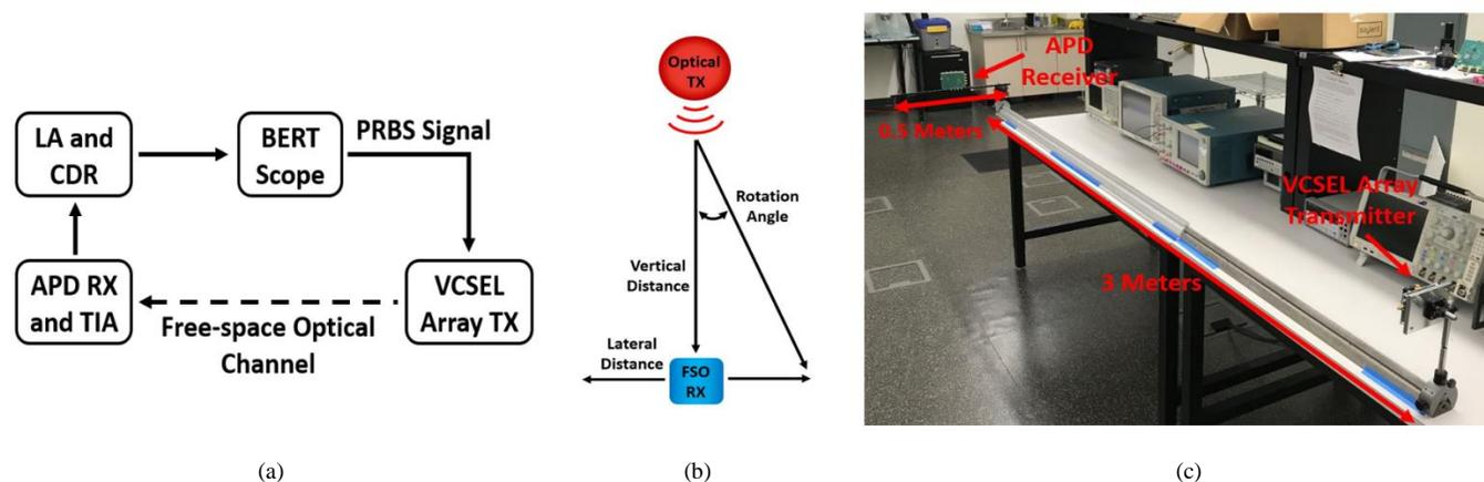
Fig. 5. FSO channel test configuration – (a) block diagram detailing the components used in the test configuration, (b) diagram showing the FSO test parameters, (c) a photo of the experimental setup showing the 0.5m optical rail mounted orthogonally to the 3m optical rail
