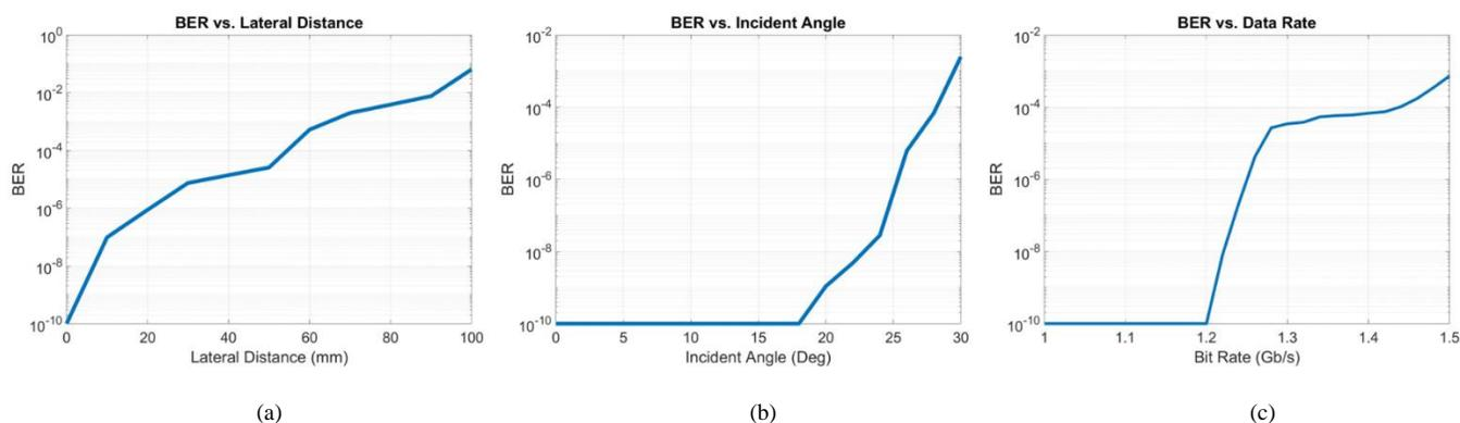
Fig. 6. FSO system BER measurements collected at a distance of 3m – (a) BER as a function of lateral motion, (b) BER as a function incident angle with respect to the optical receiver, (c) BER as a function of data throughput
