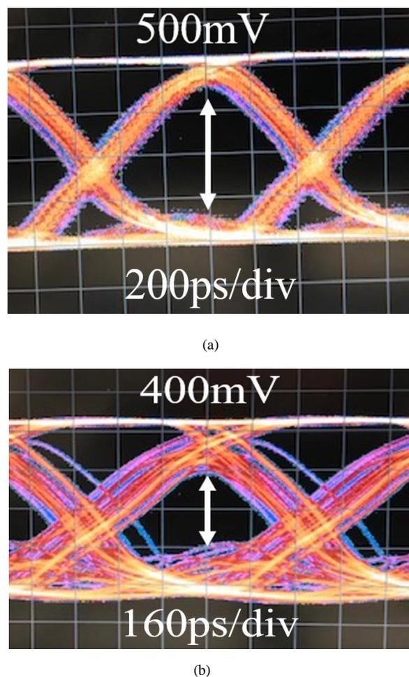
Fig. 7. Eye diagrams showing FSO signals recovered over a 3m optical channel – (a) 1Gb/s, (b) 1.25Gb/s
